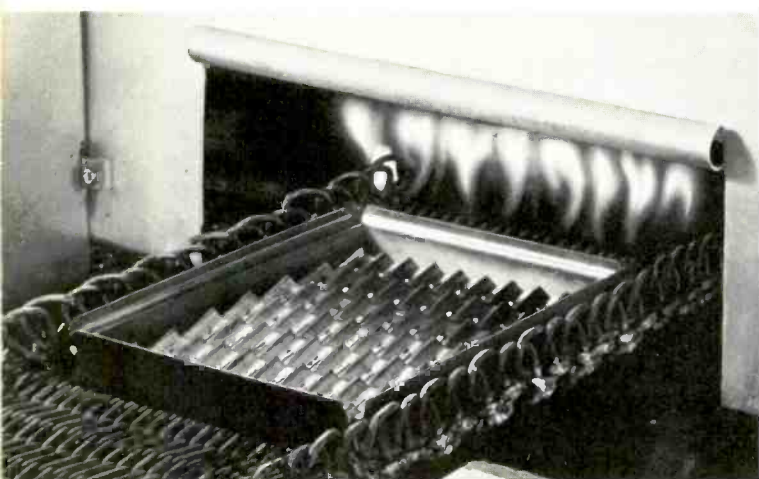
EXCLUSIVE FLAME SHIELD firing of grids and parts removes microscopic lint particles
