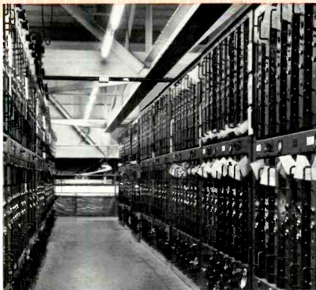
OVER 1.5 MILLION TUBES a month receive burn-in stabilization on specially designed stabilization equipment
