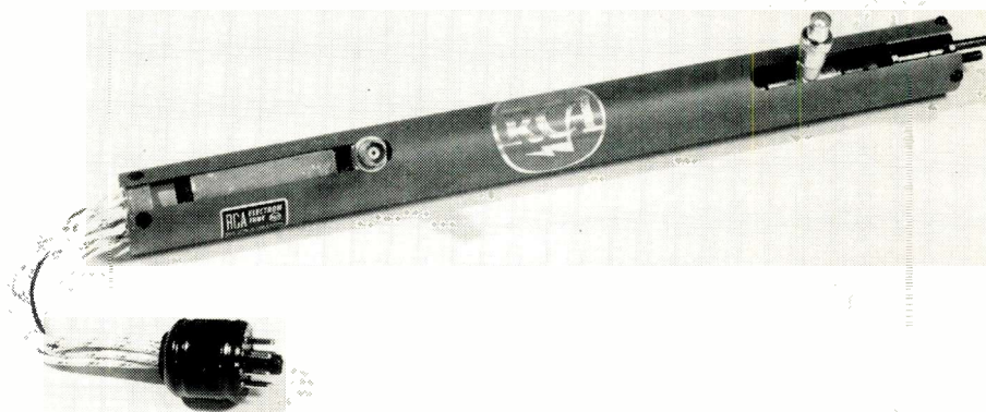
Fig. 2: The Estiatron traveling wave tube is electrostatically focused
