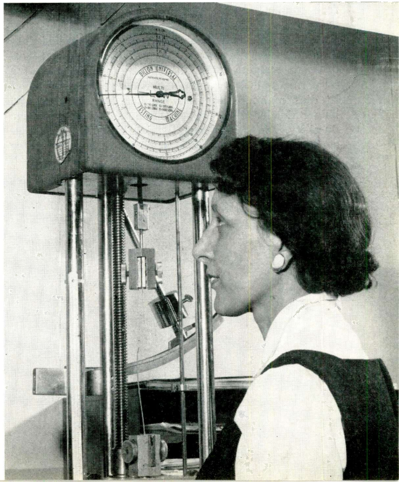
Fig. 1: The tensile tester is being used to determine the breaking strength and elongation quality of extruded Teflon.
