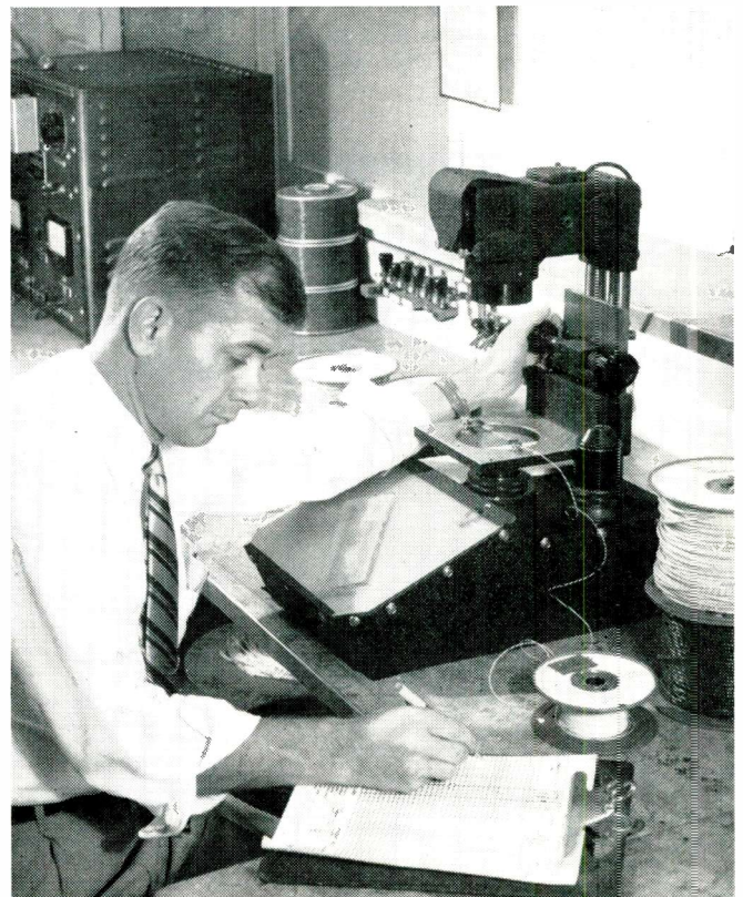
Fig. 5: An optical surface projector is used for diameter measurements and for concentricity measurements at 20X and 50X.
